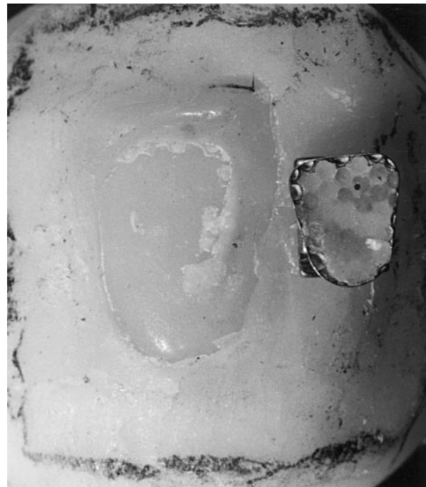
Fig 4. “Clean” cohesive bond failure. Note small amounts of adhesive remaining both on porcelain and on bracket base. No observable damage to the porcelain.
