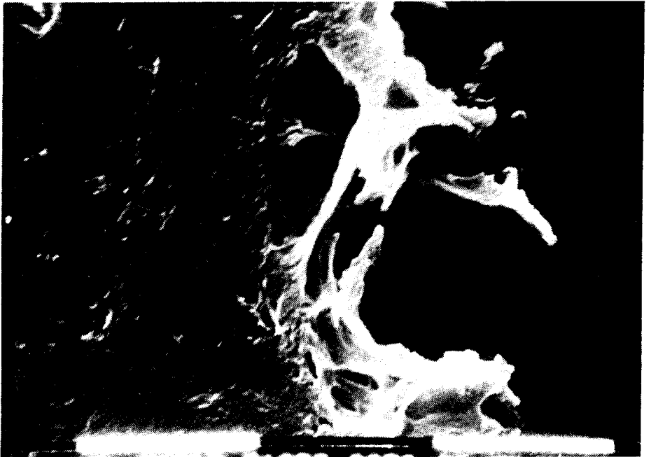
Figure 8(b). SEM picture of a cavity wall with H-Q-Bond (B) adhesive. Magnification \times 4060 .
