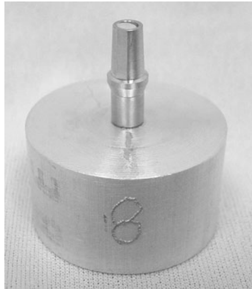
Figure 1 Stainless steel disk containing analog and attached CRC abutment.
