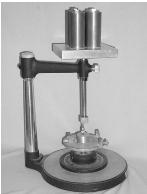
Figure 3 Modified surveyor showing 2-kg weight directed along long axis of implant at cementation.
