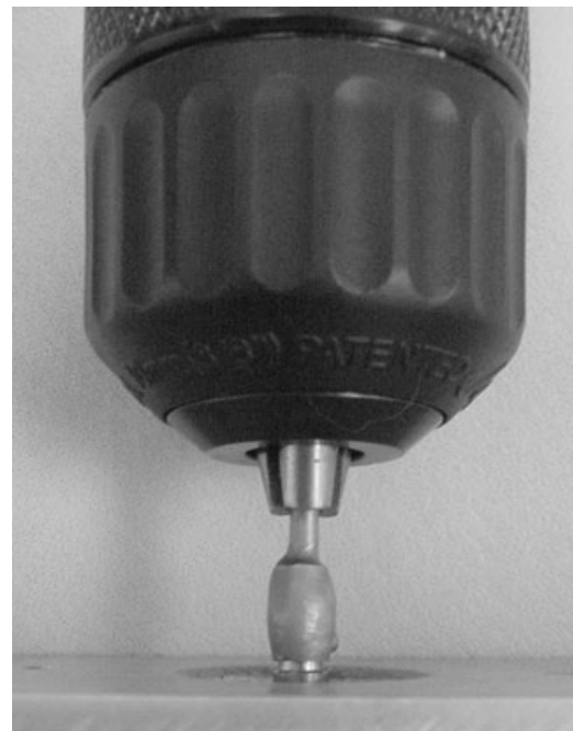
Figure 4 Disk attached to lower member and crown via sprue attached to upper member of Instron for pull-test.
